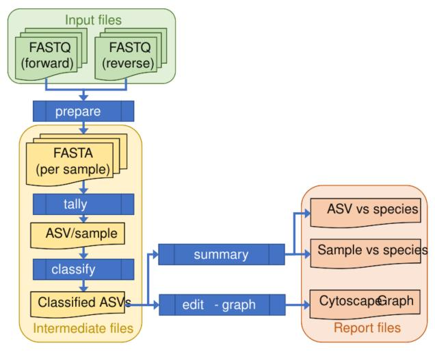
In this illustrative flow chart of the default pipeline, the input paired FASTQ files are green, the intermediate per-sample FASTA and TSV files are yellow, and the output reports are in orange. The individual steps of the pipeline are dark blue boxes.
